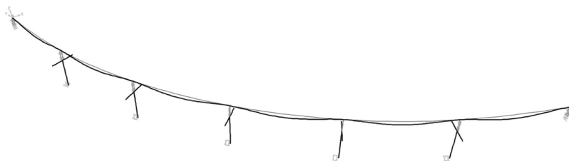
Figure 6.13 CSIBridge model after centrifugal load has been applied.
