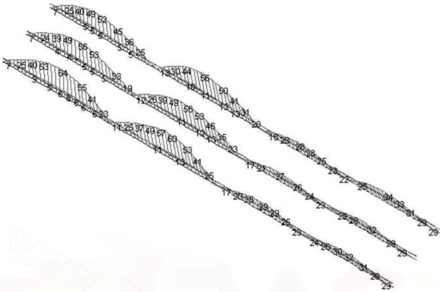
Figure 5.37 All displacements in the beam based on AASHTO, US23043 Bridge model I.
