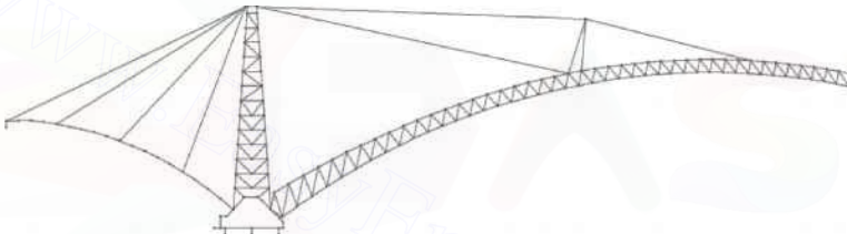
(b) Stage 2—when the half arch is lifted to half way
