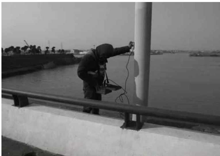
Figure 9.16 Demonstration of dynamic testing instrument on a hanger cable.
