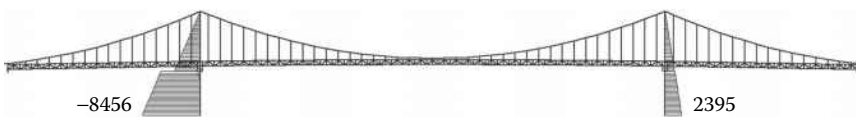
Figure 12.18 Extreme live load bending moment (kN-m) in one pylon leg of Bay Bridge.
