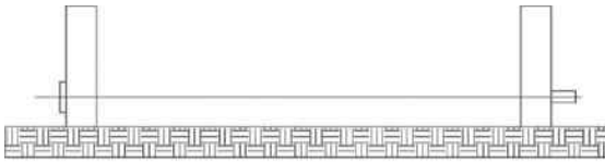
Stage 1: Tensioning of prestressing strands in stressing bed before casting concrete.
